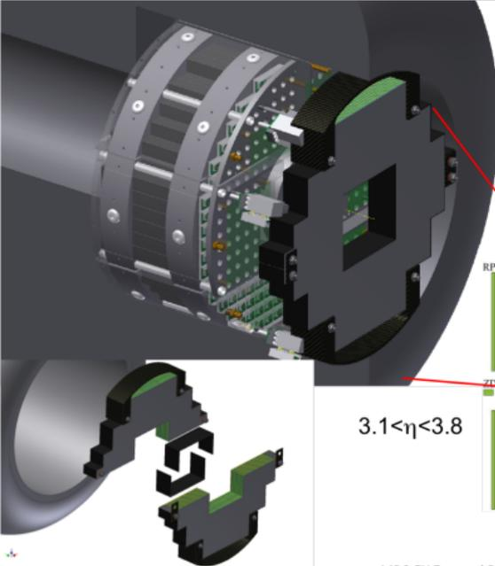
A combined charged particle tracker and EM preshower detector – dual gain readout allows sensitivity to MIPs and full energy EM showers.
